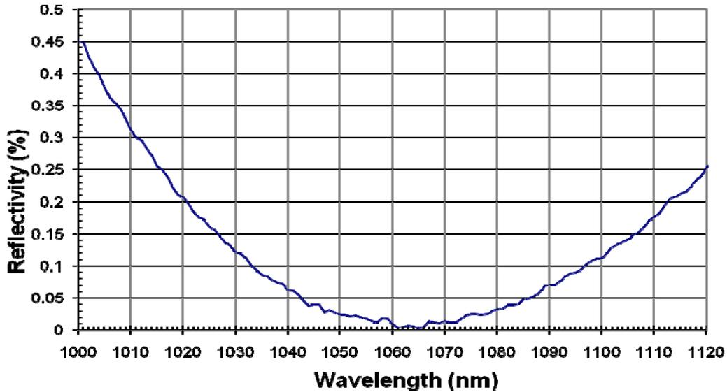
Figure 1: Measured reflectivity at  $8^\circ$  angle of incidence of AR coating fused silica witness sample
