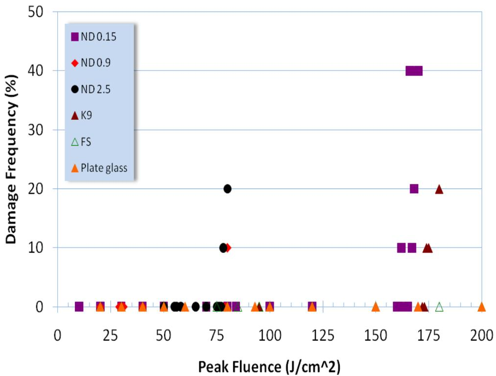
Figure 3. Laser Damage Frequency for the 6 un-coated samples.
