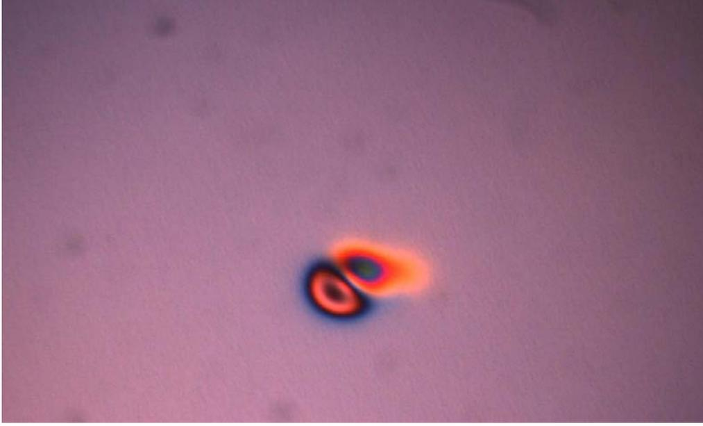
Figure 4. Image of stress induced changes in the ND 2.5 sample at fluence levels below observed permanent damage. Courtesy Spica Technologies.
