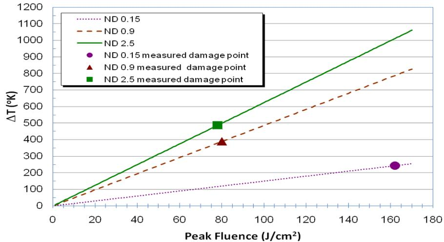
Figure 5. Estimated local heating in degrees Kelvin of the ND glass samples as function of laser peak fluence when irradiated with a single laser pulse
