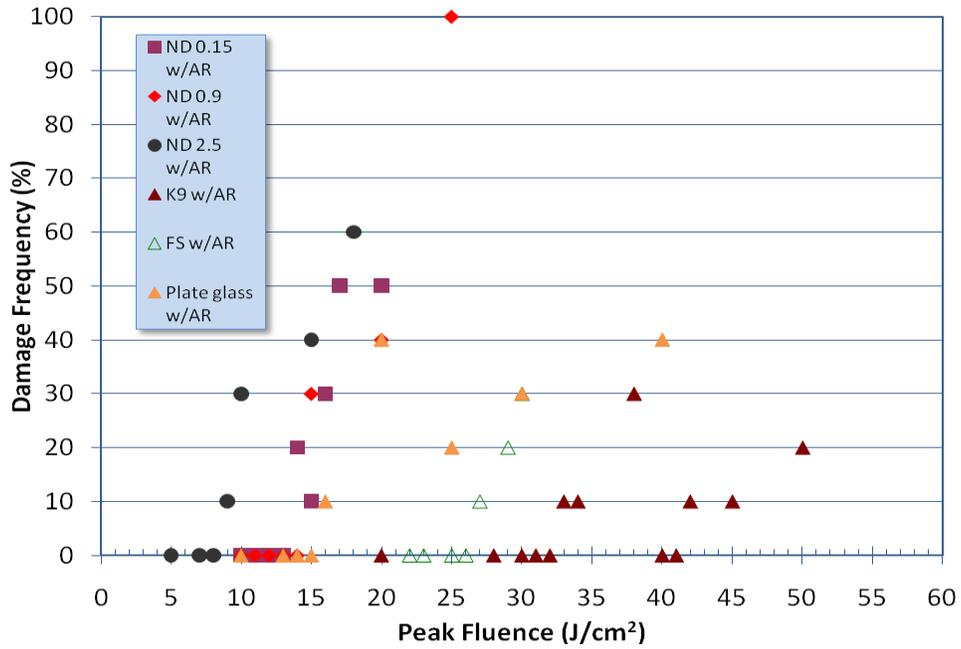
Figure 2. Laser Damage Frequency for the 6 AR coated samples.
