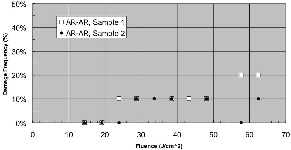
**Figure 1.** Damage site frequency as function of laser fluence for YAG samples AR coated on both sides. 10 sites tested for each fluence.
