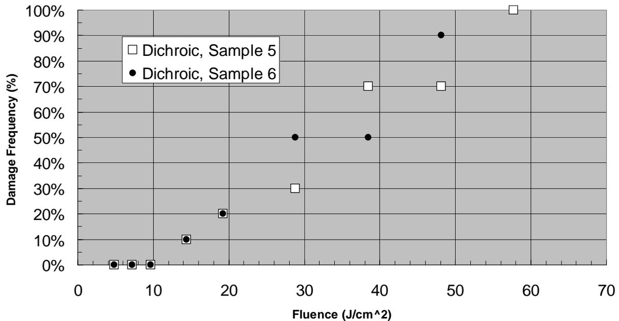
**Figure 4.** Damage site frequency as function of laser fluence for YAG samples coated with a dichroic. 10 sites tested for each fluence.
