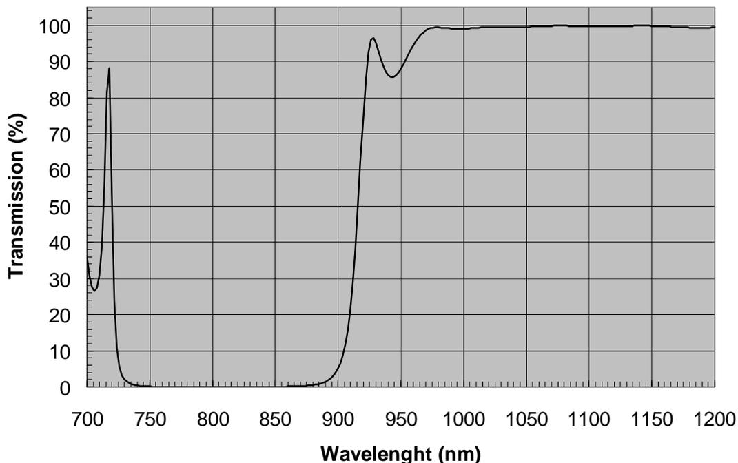
**Figure 3.** Transmission spectrum of dichroic coating on YAG. Reflection losses in the uncoated backside have been normalized out.
