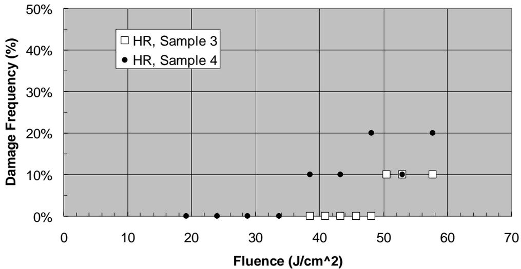
**Figure 2.** Damage site frequency as function of laser fluence for HR coated YAG samples. 10 sites for each fluence.
