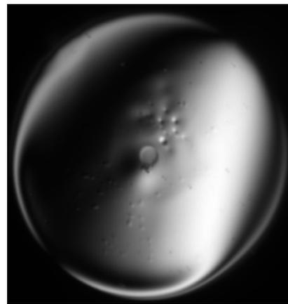
Figure 3. Example of a CO<sub>2</sub> laser-cleaved fiber showing regions with residual surface defects and undesirable surface irregularity.
