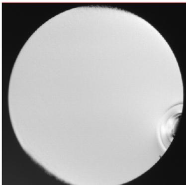
Figure 2. Example of a cleaved fiber endcap showing the typical residual chip from the cleaving process. Elimination of this chip is a delicate process that is not highly reliable.
