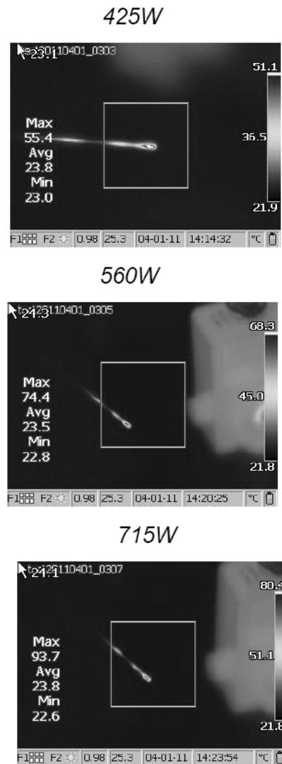
Figure 5. Thermal images of an AR coated, 4° angle-cleaved fiber endcap under operational conditions of 425W, 560W, and 715W. The CW fiber laser/amplifier system is operated at 1064nm. At 715W, the temperature of the fiber tip is ~100°C.
