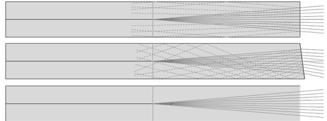
Figure 1. (top) Coreless fiber endcap fused to large mode area fiber, with the dashed lines showing back-reflected power. (middle) Same, with an angled end face on the endcap. (bottom) Same, but with an AR-coated end face on the endcap.
