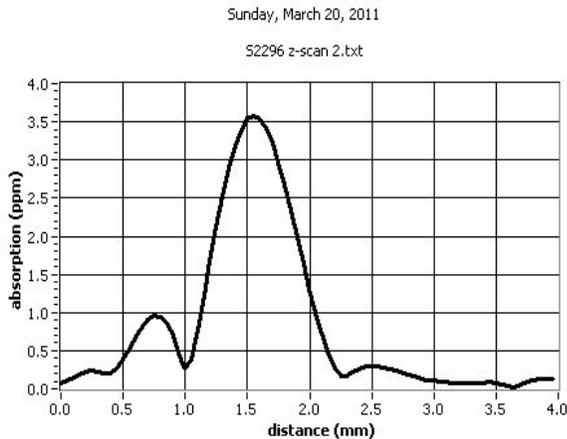
Figure 6. Absorption measurement for the witness sample from the fiber end-face AR coating run. The value for the coated surface is 3.6ppm.
