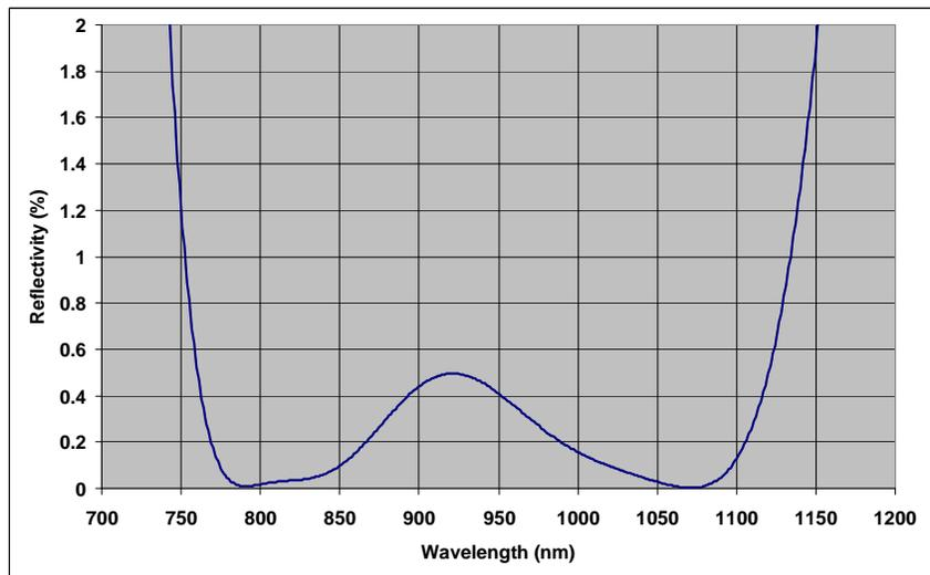
**Figure 1.** Reflection spectrum of dual AR coating on YAG.
