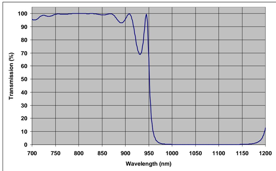
**Figure 2.** Transmission spectrum of dichroic coating on YAG.
