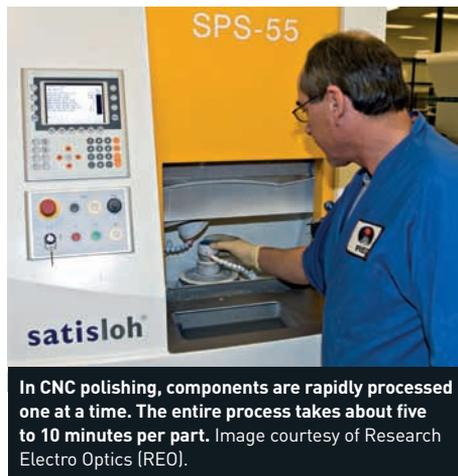
**In CNC polishing, components are rapidly processed one at a time. The entire process takes about five to 10 minutes per part.** Image courtesy of Research Electro Optics (REO).
