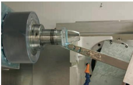
Polishing on OptiPro Systems' UltraForm Finishing (UFF) machine designed for aspheric and freeform optics.
