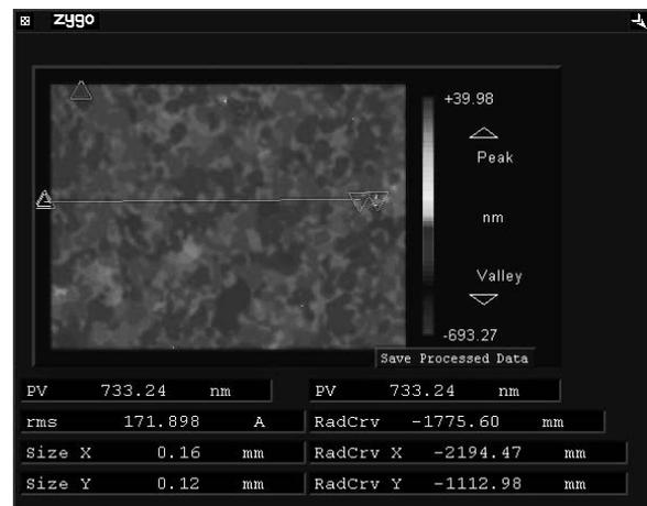
Figure 3a: Typical small aperture interferogram of polished CuW
