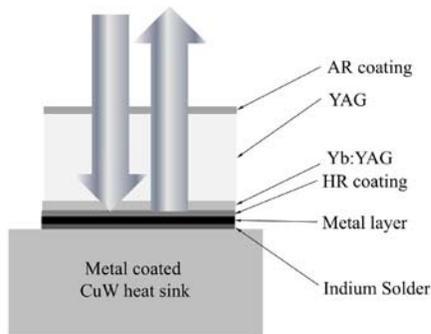
Figure 1a: Typical structure of thin disk laser soldered to CuW heat sink.
