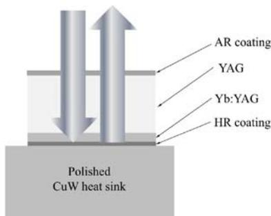
Figure 1b: Structure using CADB® direct bonding to mount the thin disk laser to the CuW heat sink
