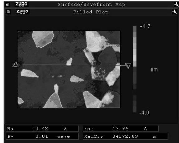
Figure 3a: Small aperture interferogram of polished Tantalum
