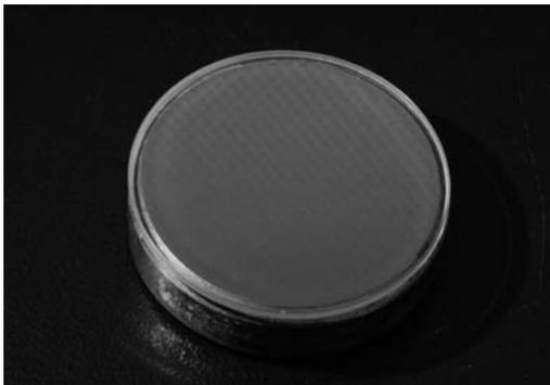
Figure 4: CADB® bonded YAG-CuW structure (sample C) with HR coating on interface.
